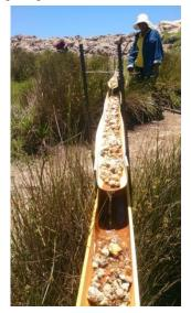
Figure 3 Carolina pilot passive treatment cascading trench
