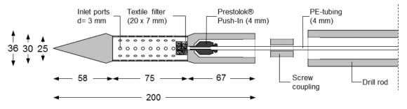
Figure 2 Drawing of the WaSP and its components (not to scale).
