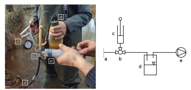
*Figure 5* Sampling equipment with the tube from the WaSP (a), a three-way value (b), the connection to the sampling syringe (c) and the air-tight collection bottle (d) with the vacuum pump (e).
