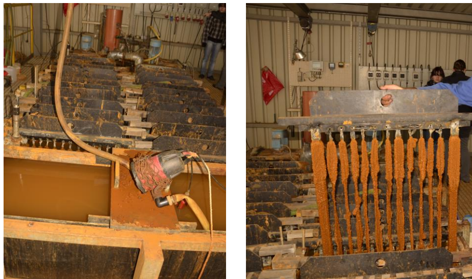
Figure 1 Treatment plant Tzschelln for the bioremediation of AMD water. The pilot plant is located at the lignite mine Nochten from which the AMD originates. Left: AMD within the oxidation basin of the pilot plant. Right: schwertmannite precipitated on carrier material within the treatment plant. (Photos: M. Mühling)
