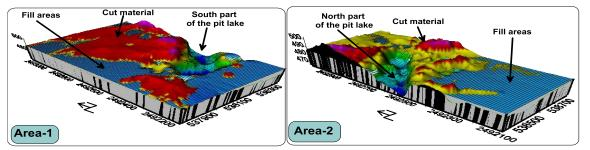
Figure 3 A simulation of cut and fill areas in Area-1 and 2 occupied by the pit lake.
