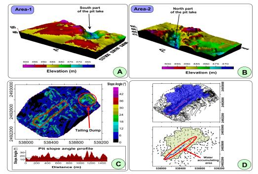
*Figure 3* (*A*) and (*B*) are the models showing the current terrain in Area-1 and 2, (*C*) is the pit lake slope analysis model, and (*D*) is an illustration of surface run-off accumulation flow to the pit lake.
