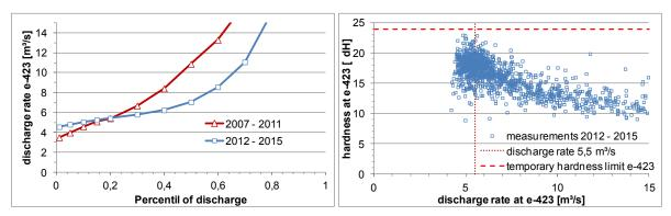
*Figure 1* Distribution of discharge before and after increase of limit (left) and the correlation of daily values of hardness measurements and discharge at measurement point e-423 in the Weiße Elster river.
