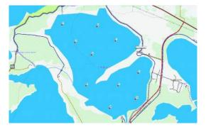
Figure 1: proposed pH network for the pit mine lake Partwitz
