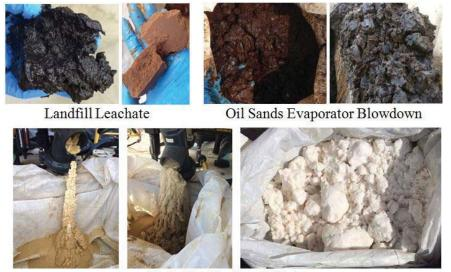
Shale Gas Produced Water Figure 8: Low Temperature Crystallizer True ZLD Solids
