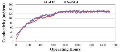
Figure 6: Achieving High CaCl<sub>2</sub> and Na<sub>2</sub>SO<sub>4</sub> Brine Concentrations
