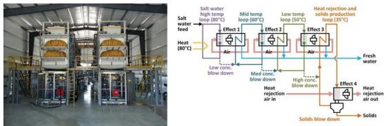
*Figure 4:* 100 m<sup>3</sup>/day Low Temperature Crystallizer (left) and Simplified PFD (right)
