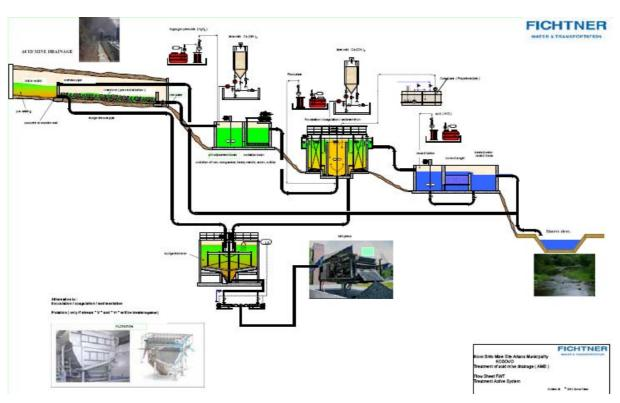
• Step 6: Sludge dewatering (thickener; dewatering)
