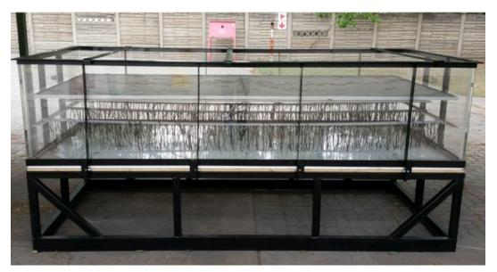
Figure 1 Image illustrating the pilot scale LFCR reactor on site, prior to inoculation
