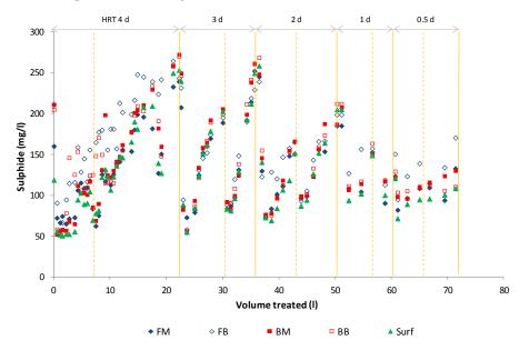
*Figure 3* Aqueous sulphide concentration at different points in the reactor as a function of HRT. Dashed vertical lines indicate biofilm collapse, while complete vertical lines indicate biofilm harvesting
