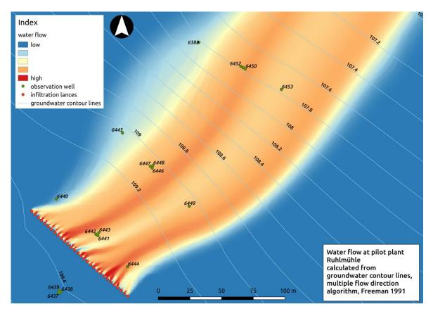
*Figure 6* Water flow at pilot plant Ruhlmühle. Shown is the direction of water flow from the infiltration lances to the stream, derived from the groundwater contour lines.
