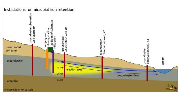
Figure 1 Vertical section through the test area.
