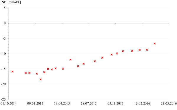
Figure 5 Increase of neutralization potential at groundwater observation well 6444.
