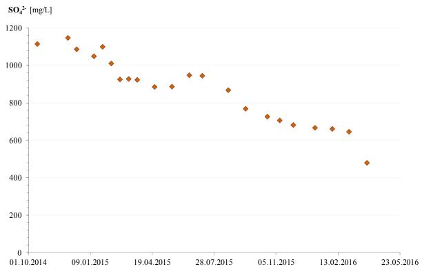
Figure 4 Decrease of sulphate concentrations at groundwater observation well 6444.
