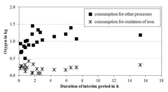
Figure 4 Dependence of oxygen consumption for iron oxidation and other processes from duration of interim period at OW 1.
