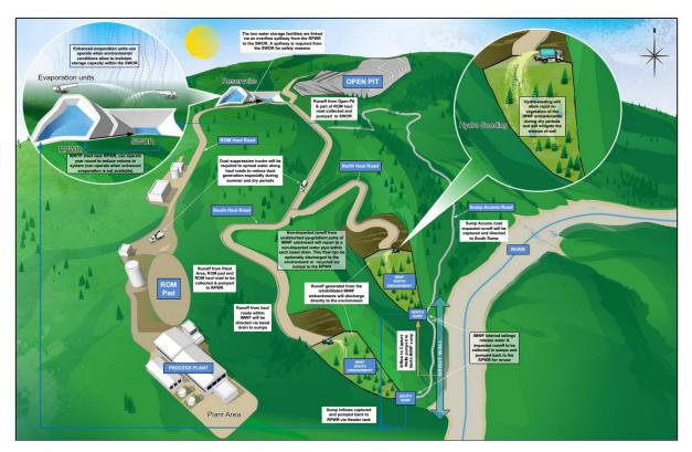
Figure 1: Schematic illustrating the challenging site water management
