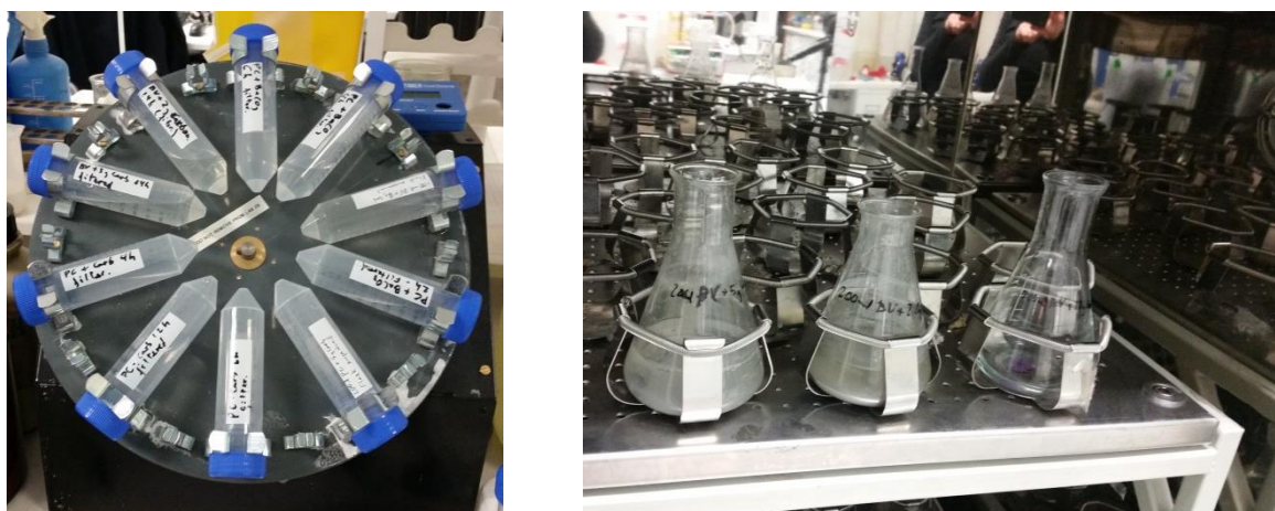
Figure 1 Pictures of batch experiments with 50 mL falcon tubes in the rotor (left) and 250 mL flask in the shaking incubator (right).
