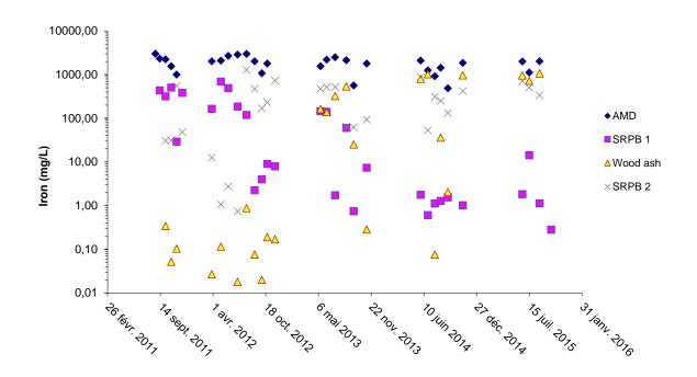
*Figure 4* Iron concentrations in each of the three-unit the passive treatment system constructed on Lorraine mine site, Quebec, Canada.
