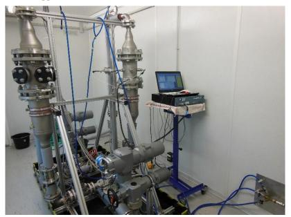
Figure 6 Test bench for in situ precipitation from geothermal brine
