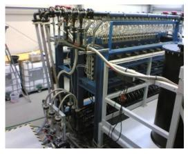
Figure 2 Uhde®-type electrolyzer
