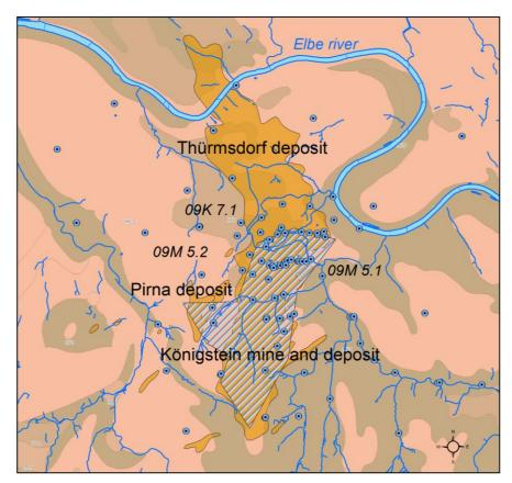
**Figure 2** Section taken from HÜK 200 (BGR 2015) with the Königstein mine (dashed area) and surrounding sub-deposits. Contour of the uranium deposit (brown) according to Tonndorf (2000). Blue spots are observation points in the 3rd aquifer. Aquifer characteristics: 09K7.1 – Quarternary gravels and sand; 09M5.1 – Turonian marlstone/sandstone, calcareous; 09M5.2 – Turonian quartz sandstone, siliceous
