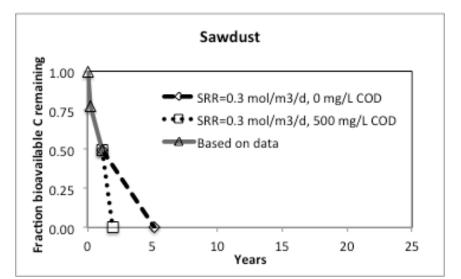
*Figure 2* Estimated bioavailable carbon utilized through 1.2 years and predicted bioavailable carbon remaining with time for sawdust under two scenarios of effluent carbon concentration and sulfate reduction rate
