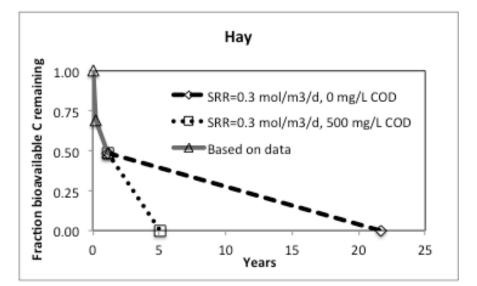
*Figure 1* Estimated bioavailable carbon utilized through 1.2 years and predicted bioavailable carbon remaining with time for hay under two scenarios of effluent carbon concentration and sulfate reduction rate.
