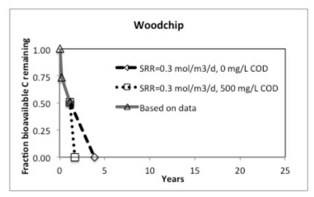
*Figure 3 Estimated bioavailable carbon utilized through 1.2 years and predicted bioavailable carbon remaining with time for woodchip under two scenarios of effluent carbon concentration and sulfate reduction rate.*
