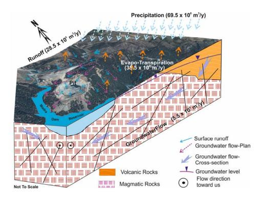
Figure 10 Block Diagram Illustrating the Hydrogeological Coceptual Model at the Mine Site.
