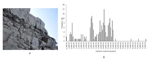
Figure 3 a) Freature Systems b) Distribution of Hydraulic Conductivity in the Mine Site
