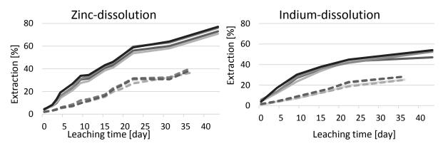
*Figure 1*: Dissolution of zinc (a) and indium (b) against time of leaching. The continuous lines show results for applications with start pH 1.6 and dotted lines for start pH 2.6.
