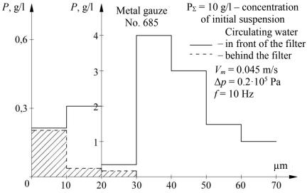
Figure 5. Efficiency of vibroacoustic waste water purification with a metal filter
