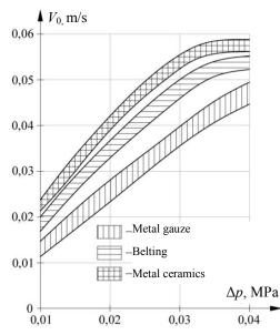
*Figure 4.* Graph of dependence of the required oscillating velocity amplitude on the type of filtering material and conditions of filtration process ( $\Delta P$ ).
