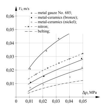
Figure 2. Hydraulic characteristics of filter materials
