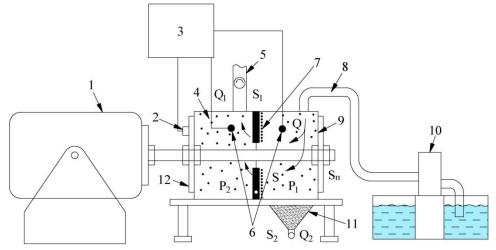
Figure 1 Schematic diagram of a vibroacoustic filter
