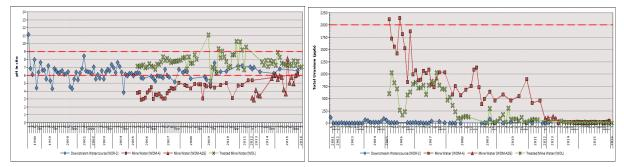
Figure 2 Temporal variation of pH and total uranium in mine water before and after active treatment and in downstream watercourse – Bica mining area
