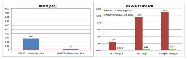
*Figure 3* Mine water PTS efficiency by comparing initial and final concentrations along treatment path (medium values in the first semester 2015) in Urgeiriça mine - Shaft4
