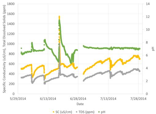
*Figure 3* Water quality at Waterloo shows a large increase in both specific conductivity (SC) and pH following unloading of the doser. The pH peaked at over 11 and SC peaked at over 1500 uS/cm.
