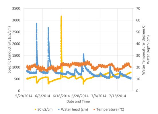
*Figure 2* Water quality at Route 56 shows the large increase in specific conductivity (SC) after the doser is unloaded on June 18, 2014. Other variations in SC at this site have a relationship with depth of water.
