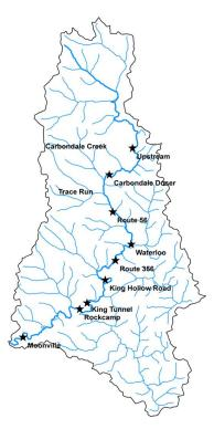
**Figure 1** Map of Hewett Fork Subwatershed located in Raccoon Creek Watershed in Southeastern Ohio. Long term sample locations are notated with black stars. The current study assesses the impact of an alkaline release from the Carbondale Doser site at Route 56, Waterloo, and King Tunnel sites.
