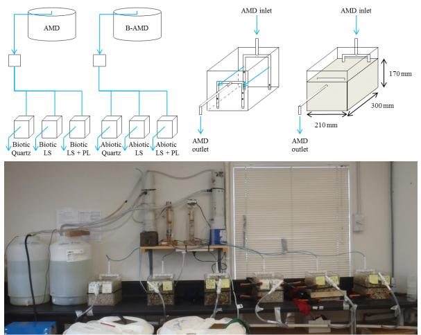
Figure 1 Experimental set up. The reactors contain: A1. Quartz, A2. Limestone, A3. Limestone and pyrolusite, B1. Quartz, B2. Limestone, B3. Limestone and pyrolusite. Reactors 1-3 receive AMD, and reactors 4-6 receive bacteriocide treated AMD (B-AMD).
