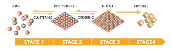
Figure 5. Scale forming process
