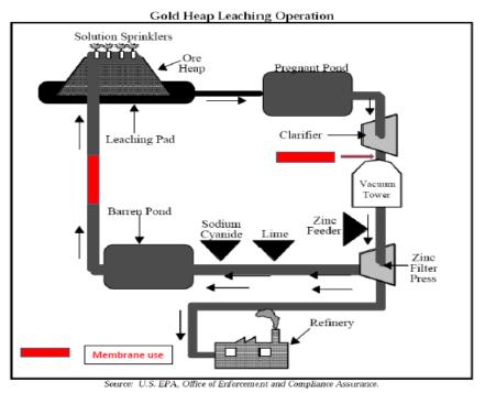
Figure 4. Membrane use in Gold leaching operation
