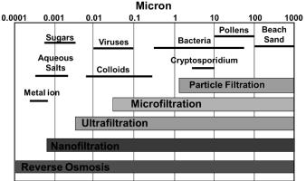
*Figure 1* Filtration spectrum of membrane processes. Courtesy of DOW Water Solutions.
