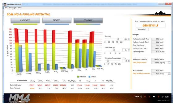
Figure 8. Genesys Membrane Master 4 scaling prediction software
