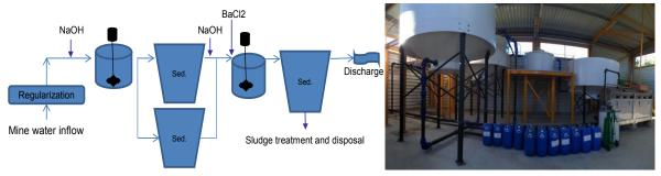
Figure 9 Cunha Baixa active treatment process and photo.
