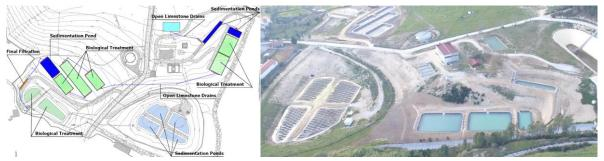
Figure 10 Cunha Baixa passive treatment process and photo.
