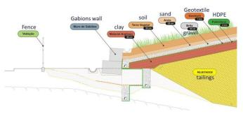
Figure 2 Multilayer cover system for radioactive mining waste confinement.
