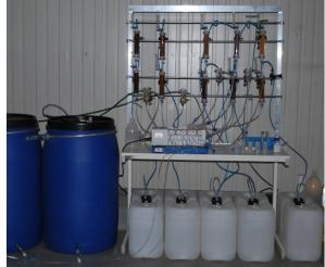
Figure 3 Pilot test setup: influent 200L-influent barrels, columns, peristaltic pump and effluent canisters
