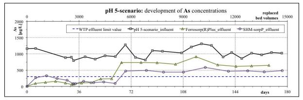
*Figure 4* Development of As concentrations in the first of each two columns filled with SHM-sorpP and Ferrosorp®Plus and seepage water pretreatment by lowering its pH from pH 8.8 to about pH 5 (pH 5 scenario: s)
