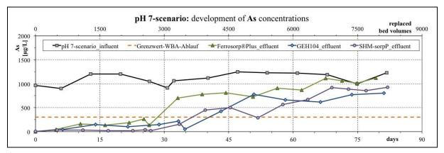
Figure 6 Development of As concentrations in the first of each two columns filled with SHM-sorpP and Ferrosorp®Plus and seepage water pretreatment by lowering its pH from pH 8.8 to about pH 7 (pH 7 scenario)
