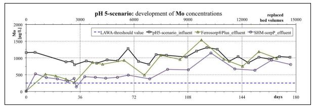
Figure 5 Development of Mo concentrations in the first of each two columns filled with SHM-sorpP and Ferrosorp®Plus and seepage water pretreatment by lowering its pH from pH 8.8 to about pH 5 (pH 5 scenario)
