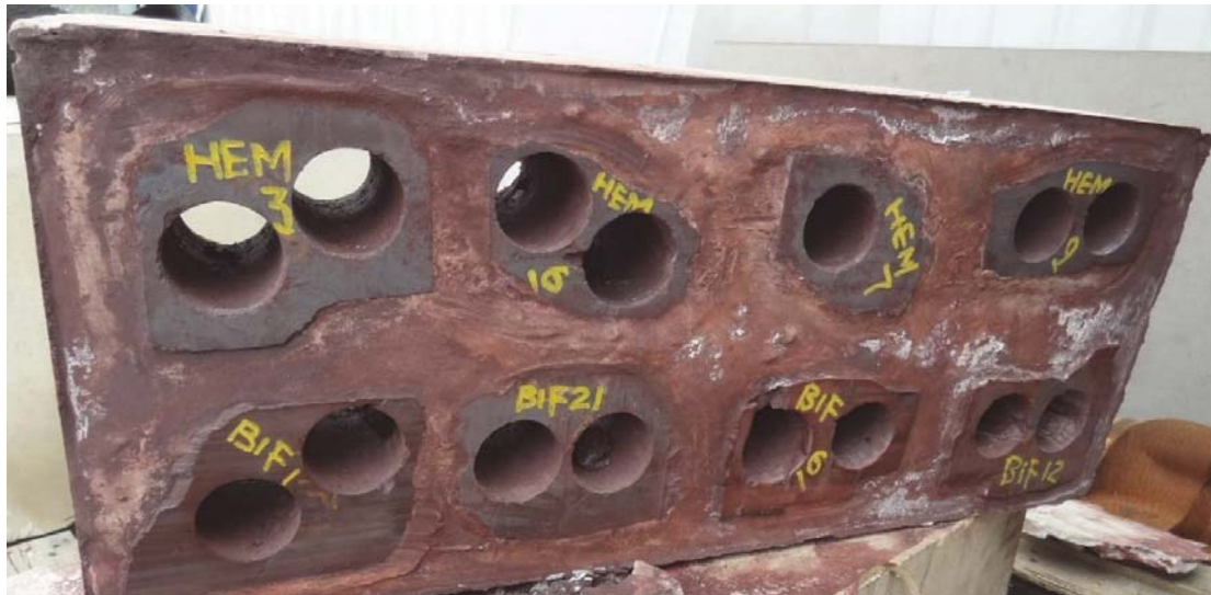
Figure 5 Laboratory drill bit testing of Sishen lithologies
