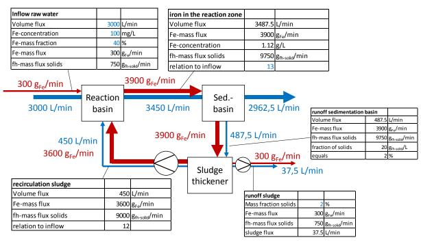
*Figure 6 Example of volume and mass fluxes of iron using the high density sludge technique (fh: Ferric hydroxide)*
