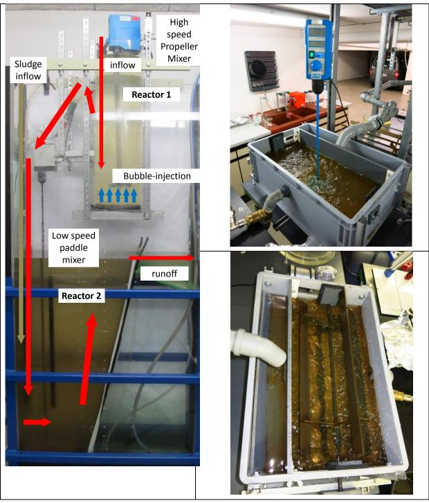
*Figure 1* Left: Bench scale plant with two coupled reactors to test the sequential influence of mixing energy input on flocculation process. Right top: Propeller mixer (405 r.p.m.). Right bottom: horizontal paddle mixer (8 r.p.m.)
