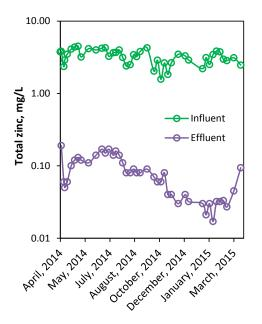
Figure 3 Zinc removal by the Force Crag mine water treatment system between April 2014 and March 2015.
