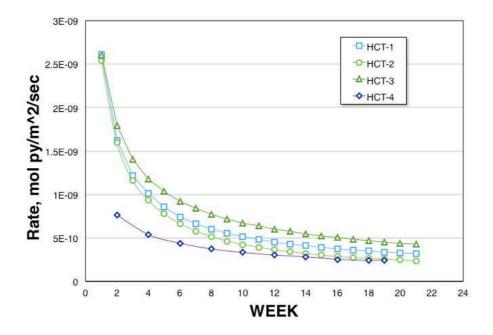
Figure 6 Rate of pyrite oxidation over time
