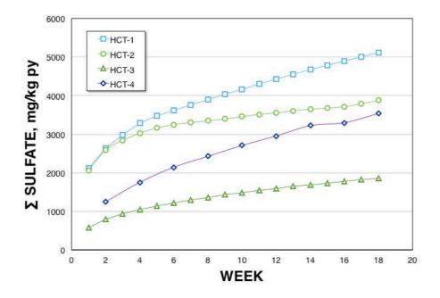
Figure 5 Cumulative sulfate production over time
