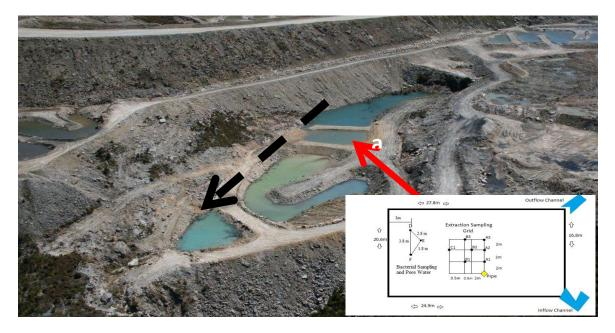
Figure 2 Emplacement of mussel shell bioreactor (location a); dashed line denotes direction of flow from the upper sediment pond, through the bioreactor and then two sediment ponds before discharge
