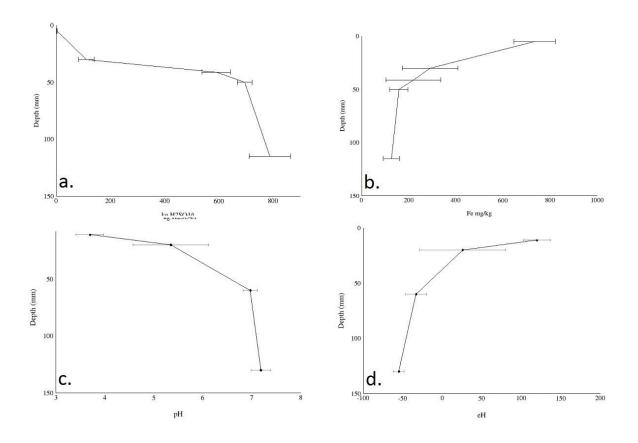
**Figure 4** A summary of the of the neutralization capacity, iron distribution pH and Eh as a function of depth for the bioreactor (a) Acid Neutralization Capacity (ANC) at different depths (mm) within the bioreactor is based on kg H<sub>2</sub>SO<sub>4</sub>/T of material (b) Distribution of total Fe(III) within the vertical depth of the bioreactor (c) and (d) show pH and Eh profiles as a function of depth in the bioreactor
