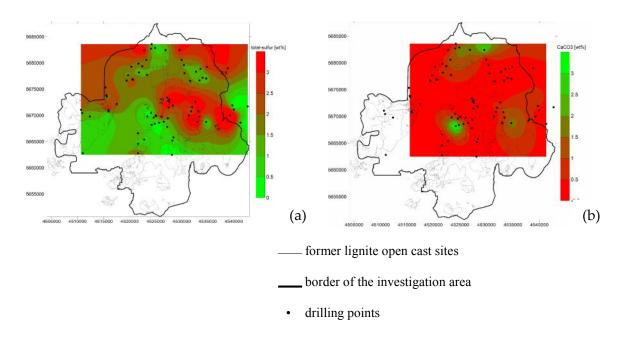
Figure 1 Predicted total-sulfur (a) and CaCO3 (b) contents (wt%) in unit 4
