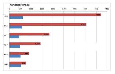
sulfate mass flow from groundwater to lake [kg/d]
