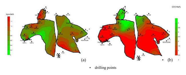
Figure 3 Predicted dump pore water composition (a) total-sulfur and (b)carbonate content in two overburden dumps
