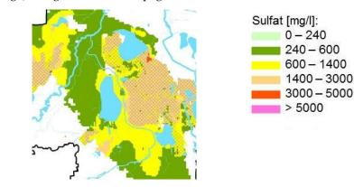
**Figure 5** sulfate concentrations in 2100 after transport modelling, aquifers 1.1-1.7
