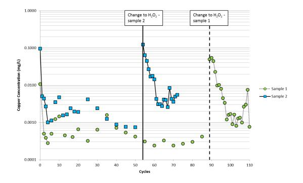
Figure 3. Kinetic test results – Copper concentrations
