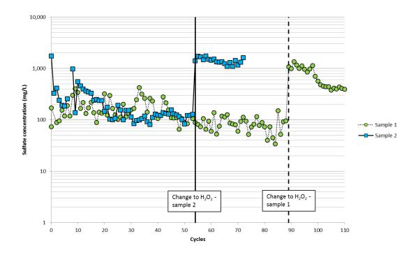
Figure 2. Kinetic test results – Sulfate concentrations
