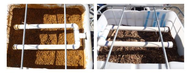
Figure 2 Adsorption chamber (on left) and bioreactor (on right) prior to being filled with water
