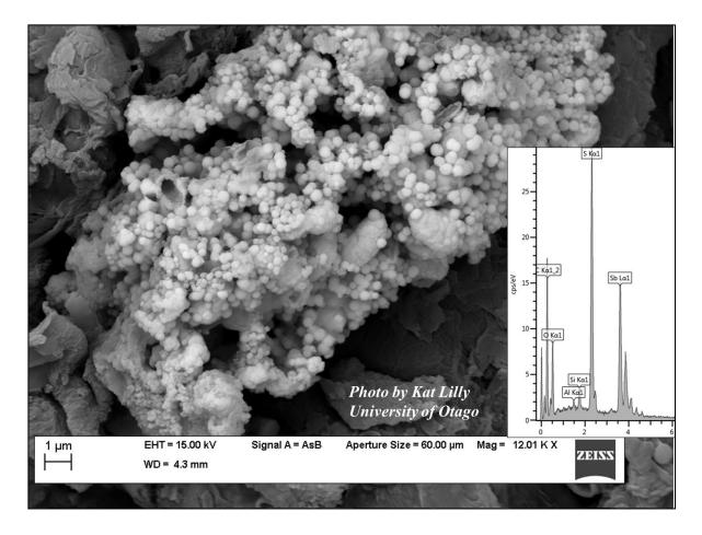
Figure 7 SEM microphotograph and EDS scan of antimony sulfide (stibnite) in substrate from the bioreactor
