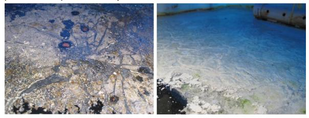
Figure 5 Precipitates on the water surface of mussel shell reactors
