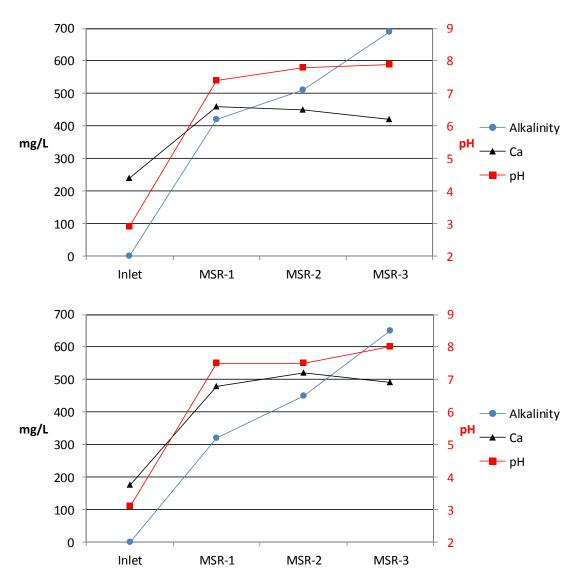
**Figure 4** Alkalinity, calcium, and pH through treatment system. **A** HRT of 56 hours. **B** HRT of 95 hours. MSR-1, mussel shell reactor 1; MSR-2, mussel shell reactor 2; MSR-3, mussel shell reactor 3
