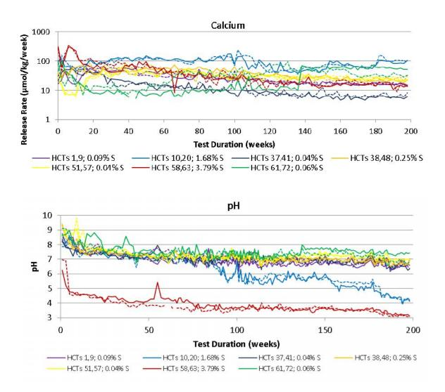
Figures 1-3 Sulfate and calcium release rates and pH for duplicate HCTs (shown by solid and dashed lines of the same color) throughout the 198 weeks of testing
