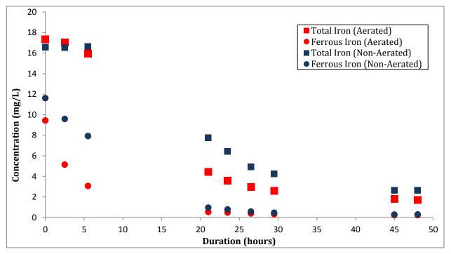
**Figure 2** Change in Fe(II) and total Fe concentration with time in column at Lindsay. Mean pH and initial DO during test = 6.58 and 8.00 mg/L respectively for aerated and 6.59 and 2.67 mg/L for non-aerated
