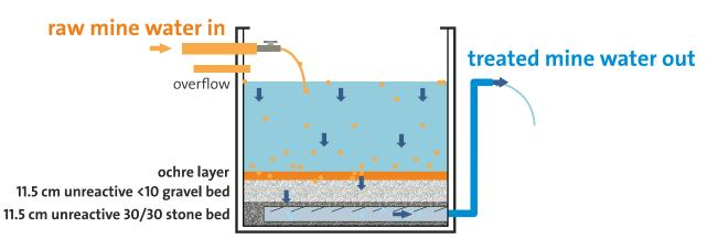
Figure 1 Schematic of Cwm Rheidol VFR
