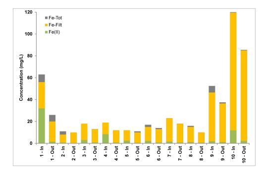
**Figure 3** Active mine site with AMD (NZ) iron concentration data for VFR influent (in) and effluent (out) on sampling occasions 1 – 10
