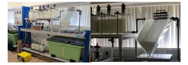
**Figure 1.** Photograph of plant in operation showing the ettringite precipitate in the clarifier and the external sludge recirculation pump in the foreground
