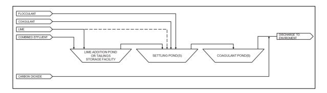
Figure 2 Base metal subsector effluent treatment model
