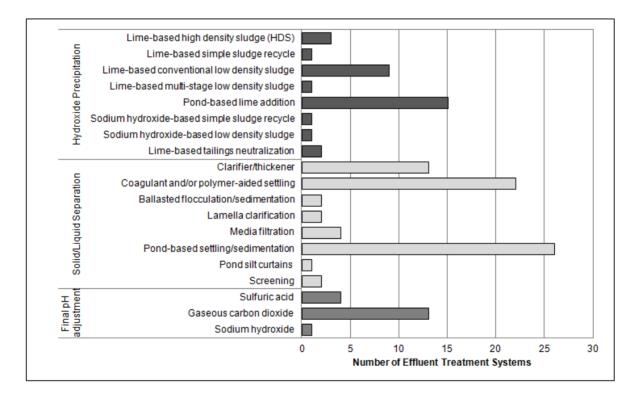
Figure 3 Distribution of hydroxide precipitation, solid/liquid separation, and final pH adjustment technologies for the base metal subsector
