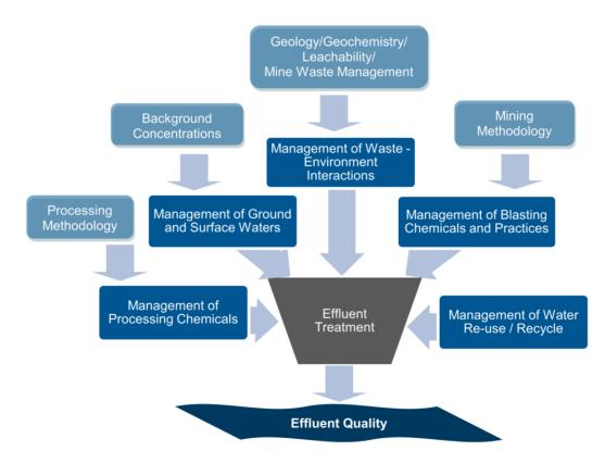
Figure 1 Factors of mine effluent quality
