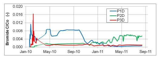
Figure 4 Bromide tracer breakthrough curves from Piles 1, 2, and 3 Lysimeter D
