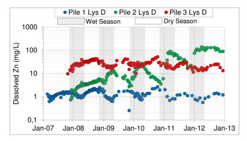
Figure 6 Dissolved zinc concentrations for Piles 1, 2, and 3
