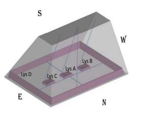
Figure 2. Schematic of the experimental piles, including three internal Sub-Lysimeters A, B, and C (4 m x 4 m) and outer Lysimeter D (36 m x 36 m).
