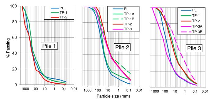
Figure 3 Waste rock particle size distributions for the protective layer (PL) and each tipping phase (TP)
