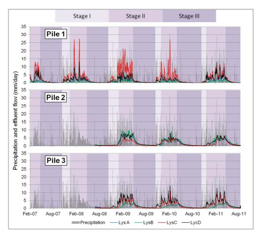
**Figure 5** Precipitation and area-normalized effluent flow from Lysimeters A, B, C, and D during Stage I (beginning of the wet season), Stage II (peak of the wet season), and Stage III (draindown and dry season)
