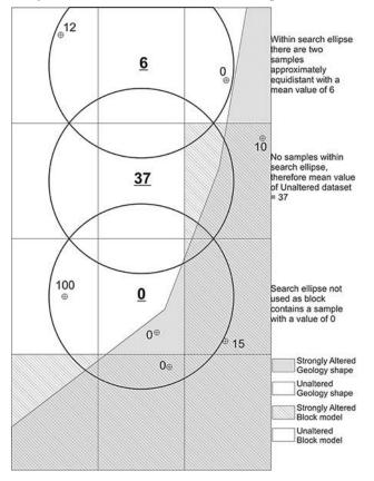
Figure 4 Conceptual diagram showing three methods for assigning a value to a block
