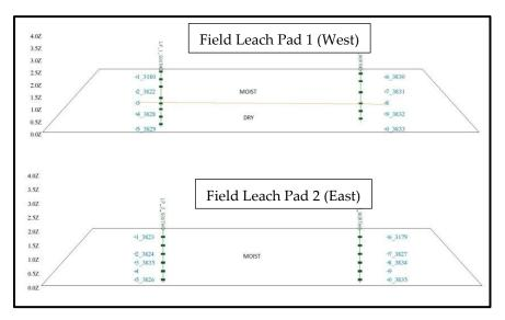
Figure 1 Field Leach Pad Sections: Green bars represent CMT ports. Blue crosses represent 650 and 229 sensors.
