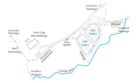
Figure 2 Schematic diagram of the treatment system at Force Crag mine (not to scale)
