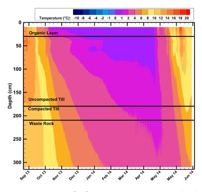
Figure 5 In situ temperature measured within the cover system and waste rock profile of cover system field trial #1.
