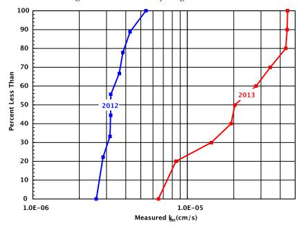
Figure 4 Cumulative histogram of Kfs values measured on compacted till layers in 2012 and 2013
