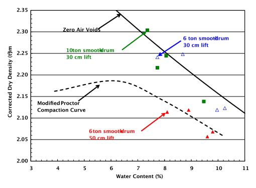
Figure 3 Comparison of dry density measurements on plateau surfaces
