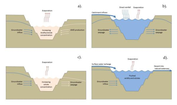
**Figure 1:** Conceptual equilibrium hydrogeological regimes for pit lakes. a) evaporative terminal sink, b) surcharged lake, c) groundwater through-flow system, d) surface water flow-through system
