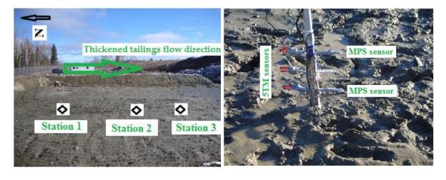
Figure 1 Experimental cell: a) Location of the different monitoring stations; b) details of instrumentation
