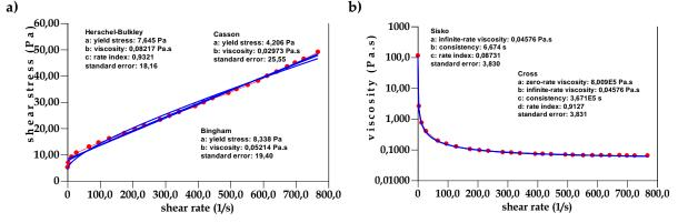
Figure 5 Merged flow (a) and viscosity (b) curves fitted with differents models
