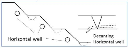
Figure 5 HDD filter well in a mine's border slope system
