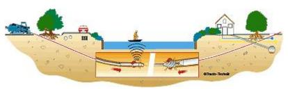
Figure 1 Schematic presentation of horizontal drilling (Tracto-Technik 2010)
