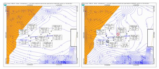
**Figure 11a)** Groundwater situation at startup of the HDD-well on 10/05/2013. **Figure 11b)** Groundwater situation 10 months after startup. Colored circles show the position of 2 observation wells.
