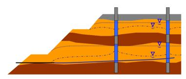
Figure 6 HDD well in connection with vertical injection well (Struzina 2012)
