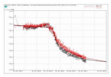
Figure 12 Comparison of observed (circles) and calculated values (line) at 2 different observation wells
