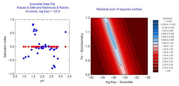
**Figures 1a,b** PhreePlot prepared figure showing saturation indices as a function of pH. The "observed" values (red dots) are all set to zero. The blue dots represent the model calculated saturation indices after the program has adjusted the log *K*<sub>sp</sub>. Figure (b) RHS, shows a contour plot showing the relationship between log *K*<sub>sp</sub> and stoichiometric value for Fe
