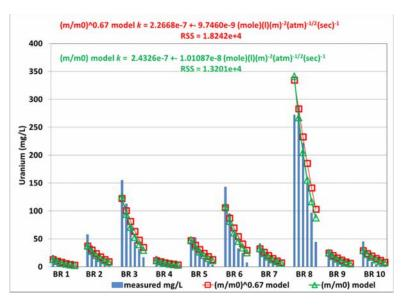
Figure 5 Bottle roll test data (blue lines) and PhreePlot Model fits. Red squares used an (m0/m)<sup>0.67</sup> term, green triangles used an (m0/m)<sup>1.0</sup> term
