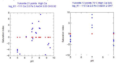
**Figure 2a**, **2b** Example PhreePlot calculations to estimate Yukonite solubility. Figure 2a (left) shows the saturation indices for the 21 samples (blue dots) at room temperature after fitting, compared to "observed" values which were set to zero (red dots). Figure 2b (right) was for 13 samples run at 75°C.
