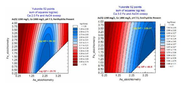
**Figure 3a, 3b** PhreePlot calculations used to evaluate stoichiometry factors for Fe and As for Yukonite. Figure 3a (left) used a Ca value of 2 and Figure 3b (right) used a Ca value of 3. White regions failed to converge in PHREEQC
