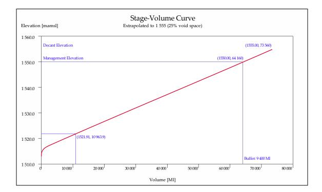
Figure 3 Stage-volume curve for the rehabilitated opencast
