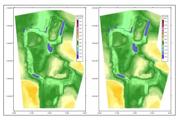
Figure 7 Flooded areas in the rehabilitated opencast - WL elevations at 1 550 & 1 555 mamsl
