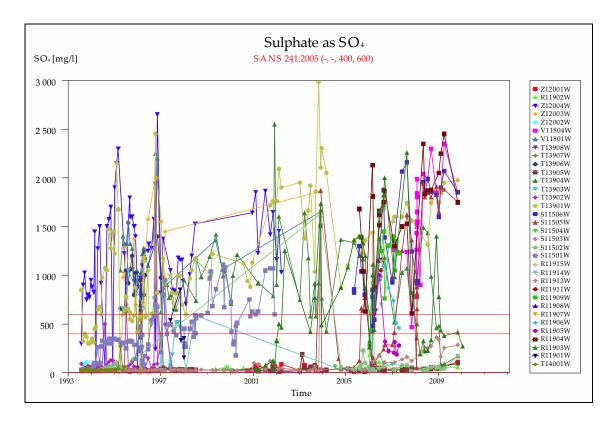
Figure 9 Recorded sulfate concentration at the colliery
