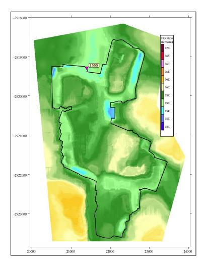
Figure 2 Opencast surface contours with decant point indicated
