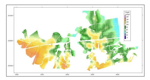
Figure 4 Depth of the coal floor in the current and future underground sections of the colliery
