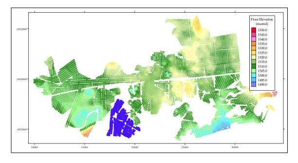
Figure 5 Coal floor contours for the current and future opencast and underground workings
